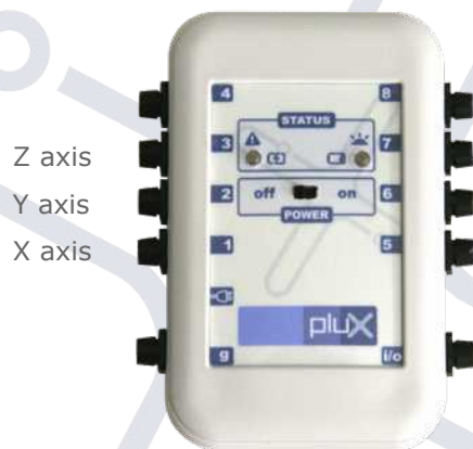
Figure 3: xyzPlux suggested connection
